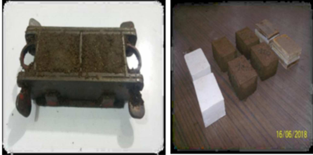
Figure 4. Molding and demolding of three characterized insulating materials.
