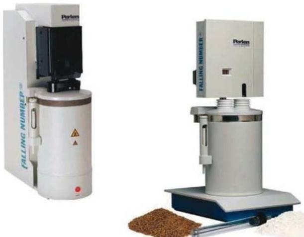
Figure 19. Falling number machine.
