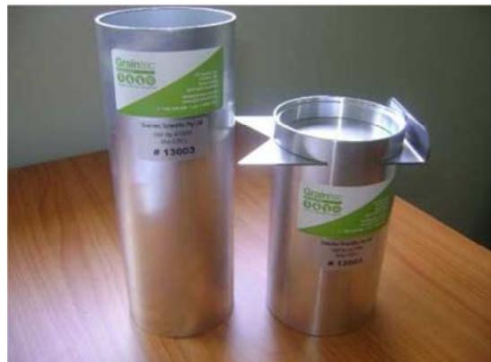
Figure 18. Hectoliter test weight kit.
